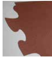
Prepreg (Preimpregnated) carbon or glass fibers in non-hardened duroplastic matrix.
