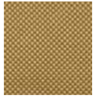
Aramid fiber (Kevlar™) Synth. Polyamid-fiber in woven, non-woven, unidirectional form.
