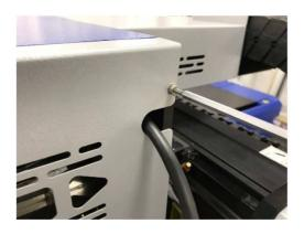
2. Clamp the ink line with the red clamp for the head you are about to flush The LXiR series does not have head clamps, when you untwist the ink lines you will hear a clicking noise until you attach the syringe connection
