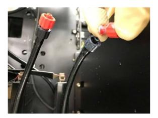
5. Connect the syringe the and slowly push the cleaning solution through the head.
