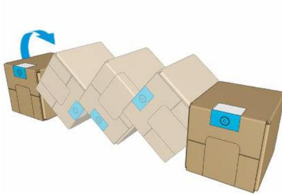
For the White cartridge, shake it 60x times while rotating it to ensure it will be well mixed.
