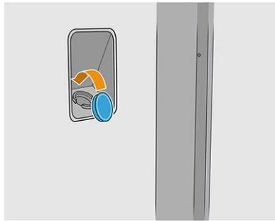
c. Open the carriage cover and tap the **Purge** button to fill up the water dispenser system. The cleaning roll will advance 5.08 cm (2 inches) and some water will be purged on the cloth. If no water is present in the cloth, tap again the **Purge** button until the water is fired.
