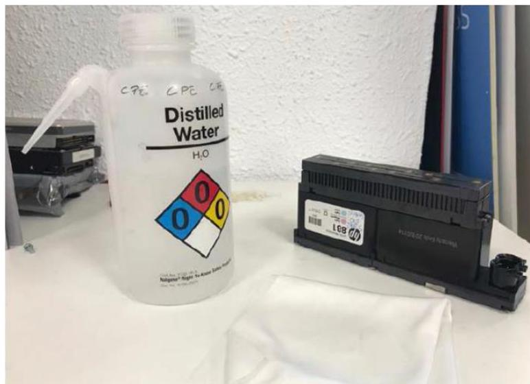
2. Place enough distilled water (a couple of drops should be enough) to cover the nozzles completely and allow some time for the water to soften the ink.
