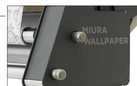
Front rewinding shafts with independent clutches
