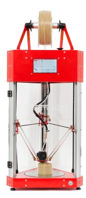
The T650P (PEEK) is our very own high temperature 3D printer. Its nozzle can reach a temperature of 450 degrees Celsius and its build plate goes up to 175 degrees Celsius. This, alongside its closed chamber to ensure better temperature stability, allows you to print with high temperature materials such as PEEK and PEI/Ultem™.
